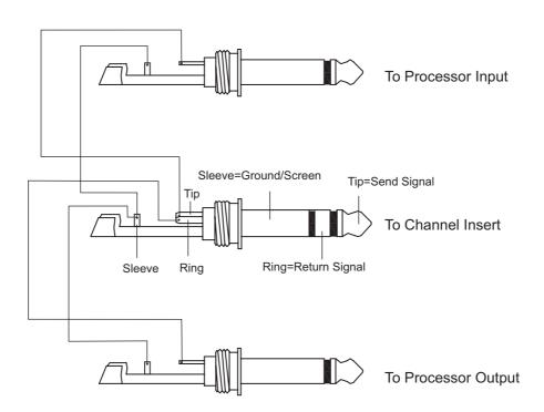
$\rm Y\,\text{-}Stereo$  lead for insert Connection (To be used when the processor does not employ a single jack connection for the In/Out Connections)
